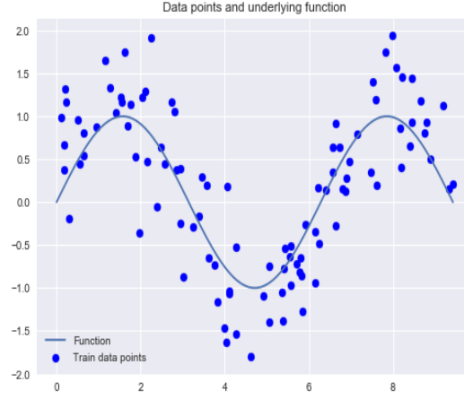
Figure 2.11: Data set generated by a sin function, with added Gaussian noise.
