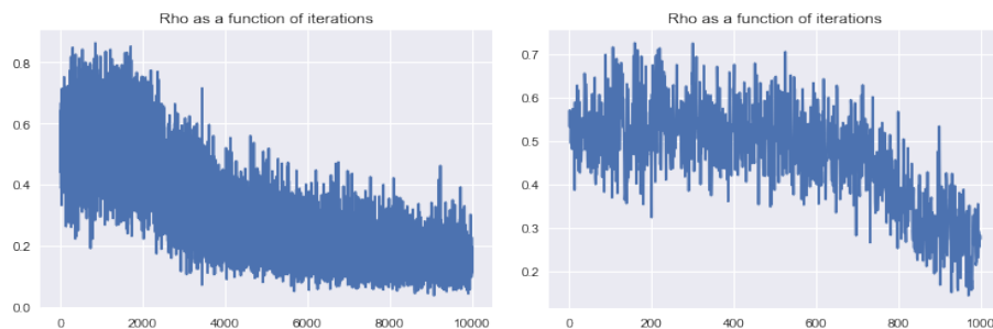
Figure 5.2: The value of \rho over time, for 10000 iteration with batch size 100 (left) and 1000 iterations with batch size 300 (right).
